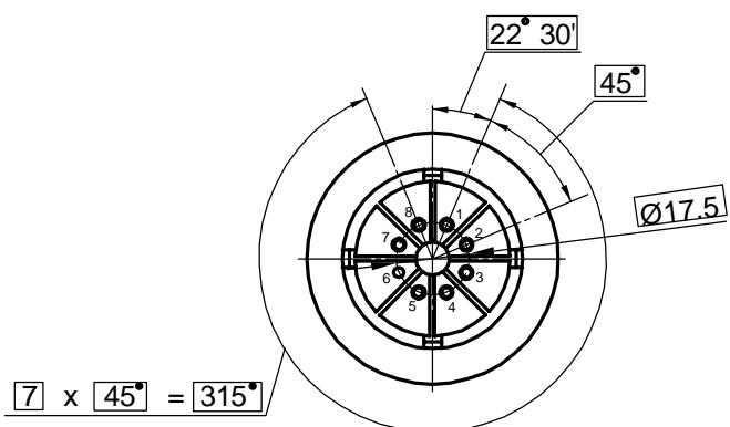
Electrode -to - lead connection diagram
